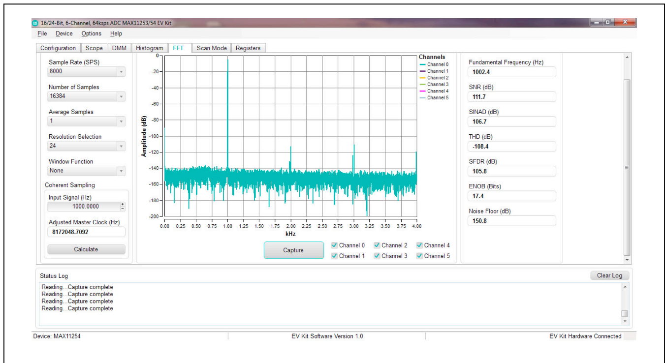
Figure 5. EV Kit Software (FFT Tab)
