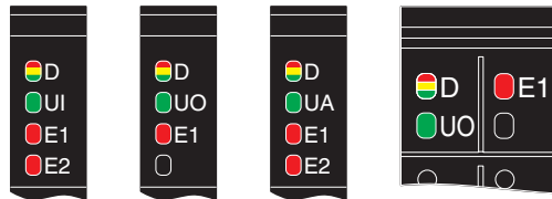
Figure 8-2 LEDs on the power connectors (examples)
